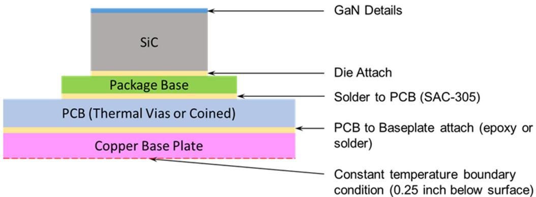
Figure 3. Thermal Model Stack-up for TGA2307-SM EVB.
