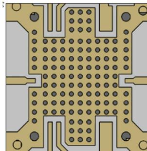
Figure 1. Mounting detail for the TGA2307-SM EVB PCB.
