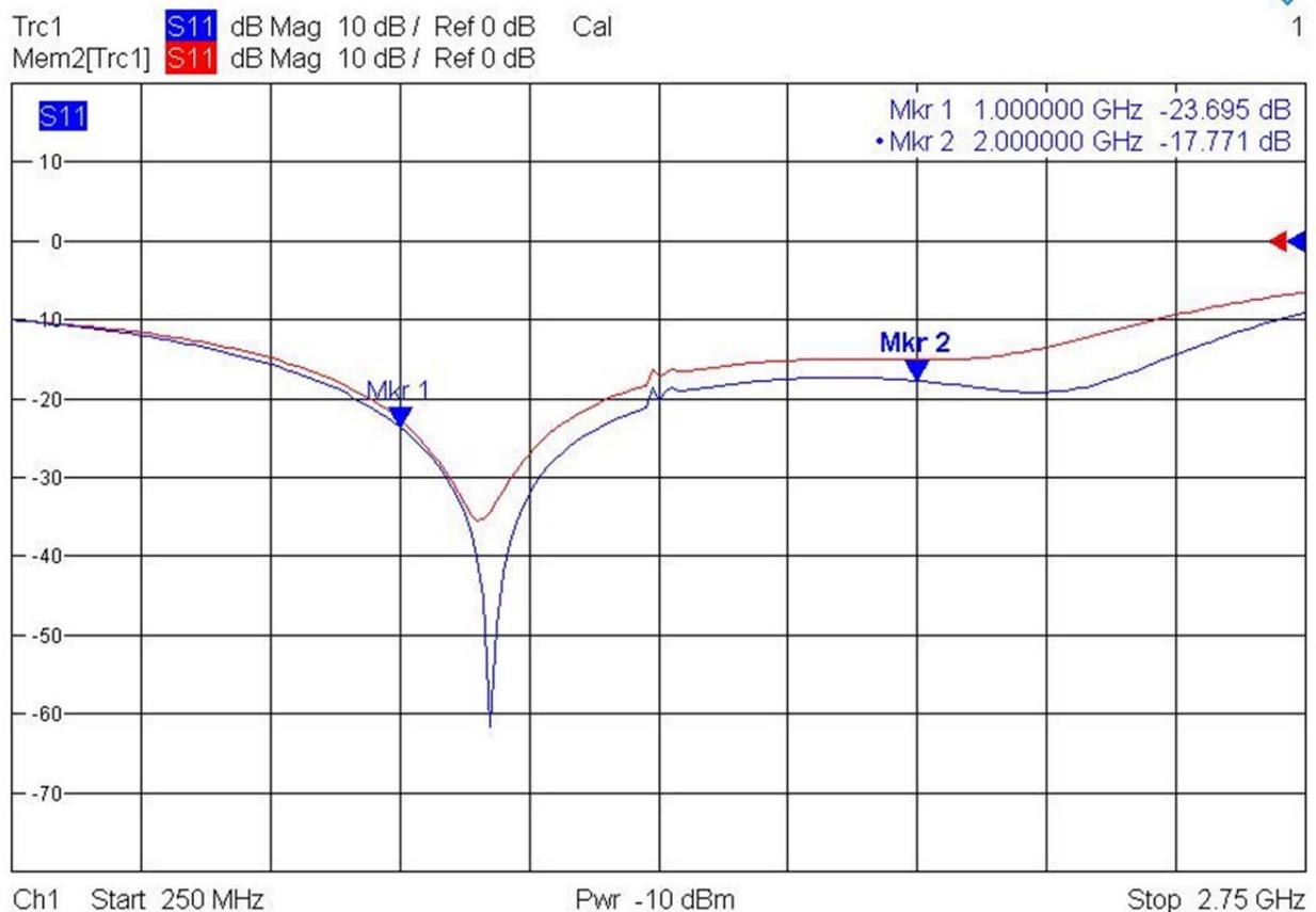
It can be seen that this configuration gives a good wideband input return loss, better than 15dB from 750MHz to over 2000MHz.
