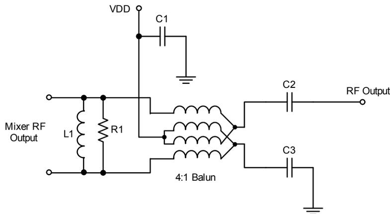
The 4:1 balun fitted as standard on the evaluation boards is the RFXF8553 transmission line transformer, covering 500MHz to 2500MHz. This part actually operates down well below the specified frequency of 500MHz. An alternative for lower output frequencies is the RFXF6553 transformer covering 10MHz to 1900MHz. The secondary center tap of the transformer is used to provide the mixer DC supply.
