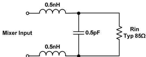
The resistance term  $R_{IN}$  will be approximately 85Ω at the default mixer current setting (100). The following table shows how the resistance varies with mixer current setting.
