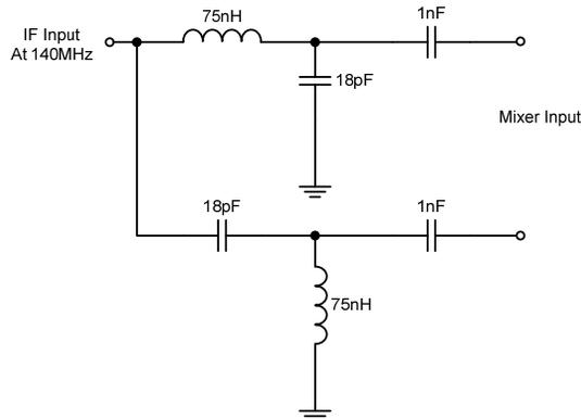
The following table shows balun components calculated for different frequencies, and rounded to the nearest standard component value. The conversion is 50Ω:85Ω, to match to the real part of the mixer input impedance.
