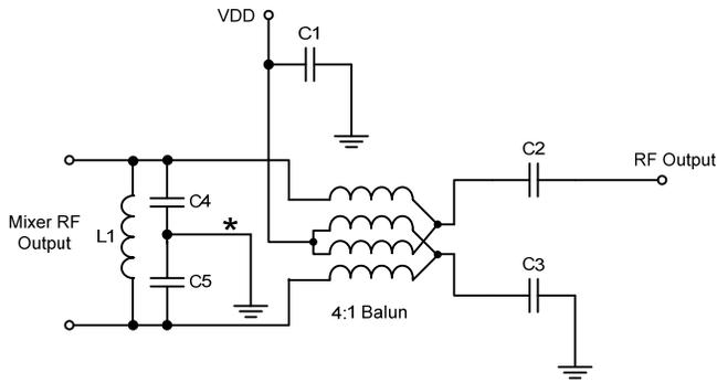
\* Note that alternatively this point could be taken to the VDD power plane. The power plane will then require suitable high frequency decoupling to the ground plane.
