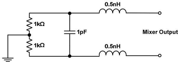
The mixer output does not need a typical conjugate match; it just needs to see a resistive load. The mixer output sources constant current, so a higher load resistance will give higher output voltage and gain. A shunt inductor can be used to resonate with the mixer output capacitance at the frequency of interest to improve the conversion gain. This inductor may not be required at lower frequencies where the impedance of the output capacitance is less significant.
