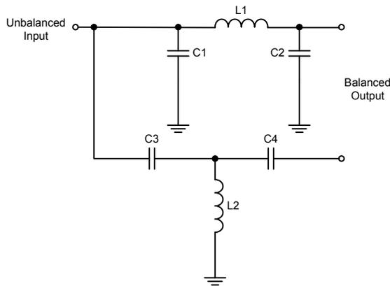
The lead and lag elements could also be achieved using quarter wavelength transmission lines in microstrip. This is not a very practical solution at these frequencies due to the physical size.
