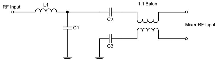
The 1:1 balun is the RFXF9503 transmission line transformer, covering 5MHz to 3000MHz.
