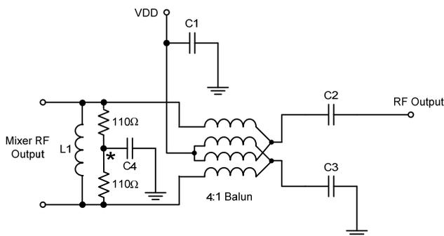
\* Note that this point could be taken to the VDD power plane. The power plane will then require suitable wideband decoupling to the ground plane.
