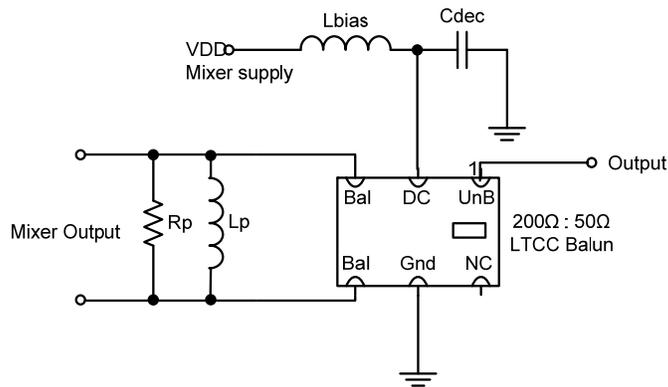
For the RFFC507x mixers a different approach is required when the output frequency is above approximately 4500MHz. The output capacitance of the mixer becomes increasingly difficult to match with a shunt inductor, especially since the output bondwires contribute significant inductance of 0.5nH each. It is recommended to lower the output impedance by using a 50Ω:100Ω or 50Ω:50Ω balun, or by using the shunt resistor  $R_p$ . Further information is contained in a separate note, see Reference 2.
