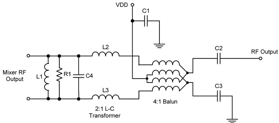
Note that L2 and L3 conveniently carry the mixer DC supply to the output pins. In this case R1 would be 510Ω, giving 400Ω in parallel with the mixer output resistance. The values of the L-C components in the 2:1 transformer, and the parallel inductor L1, need to be adjusted to give the best output match combined with the mixer output capacitance.
