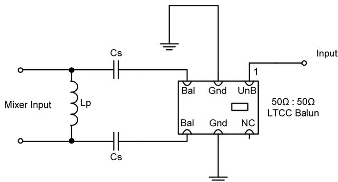
Since the mixer input impedance real part is around 85Ω, dependant on frequency and current setting, a 100Ω:100Ω balun could be used and the matching circuit changed accordingly.
