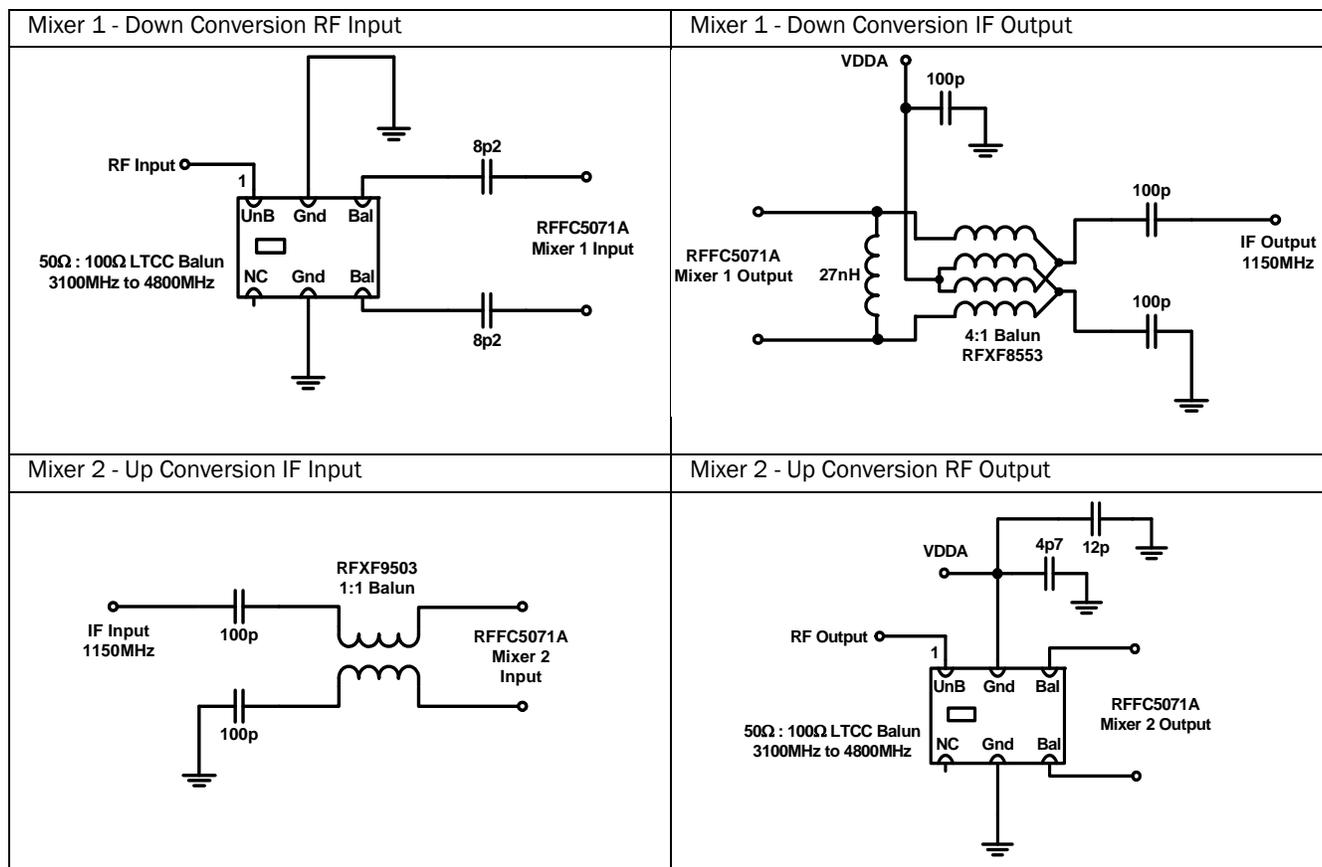
Note: The results overpage are measured between SMA connectors on the FC5071A410(A) evaluation board, BOM modified as shown above. The results include all balun and PCB losses.
