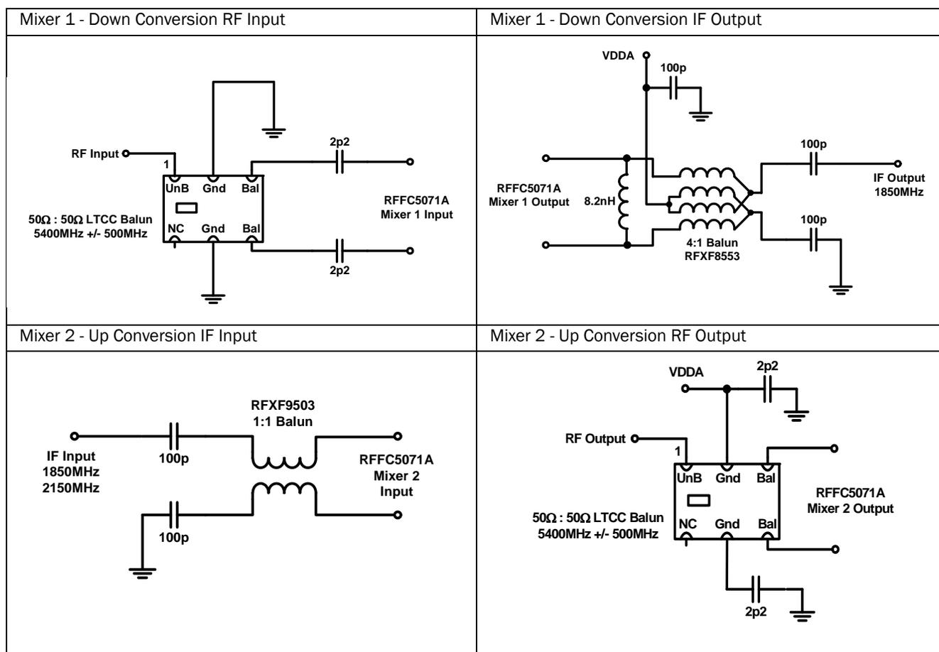
Note: The results overpage are measured between SMA connectors on the FC5071A410(A) evaluation board, BOM modified as shown above. The results include all balun and PCB losses.
