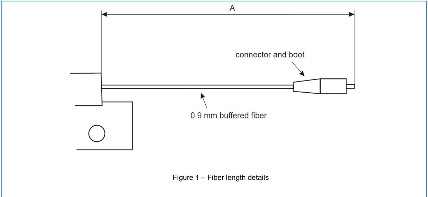
Package Drawing (Dimensions in millimeters)
