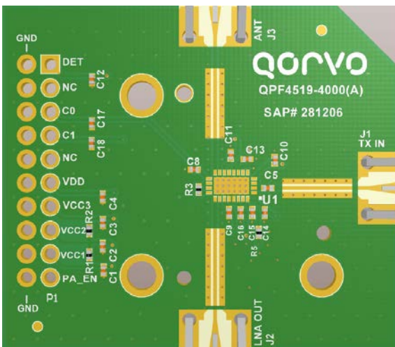
Figure 2a. QPF4519 Evaluation Board Photo
