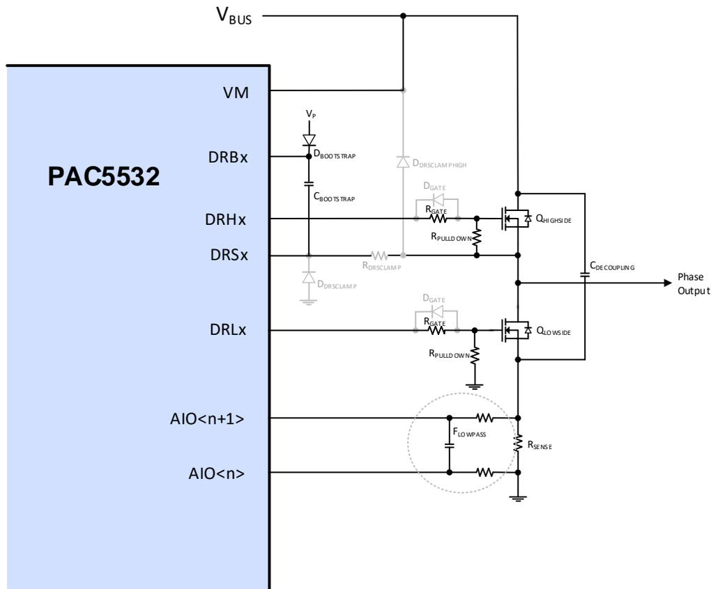
The value of the current sense resistor ( $R_{SENSE}$ ) is selected based on the power requirements of the application.  $R_{SENSE}$  should be placed as close as possible to the Low-Side Power FET ( $Q_{LOWSIDE}$ ).
