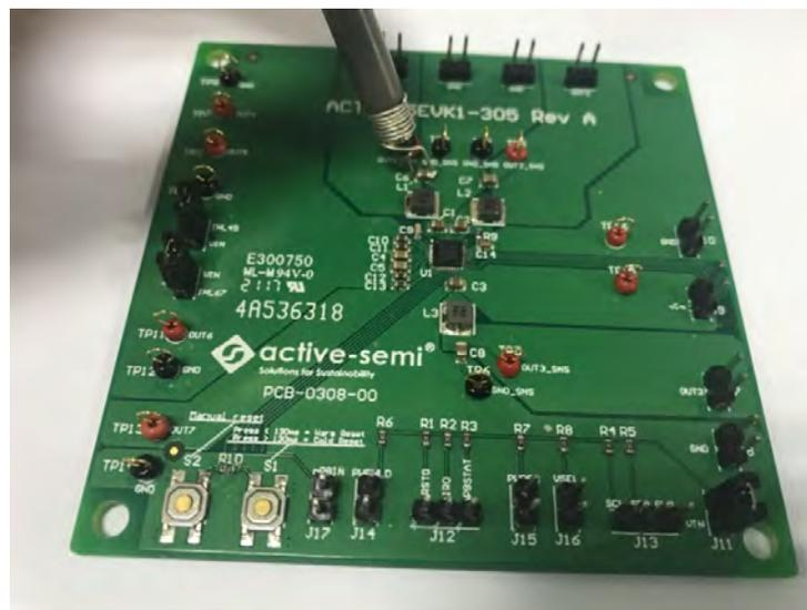
**Figure 4—Measuring output voltage ripple**
