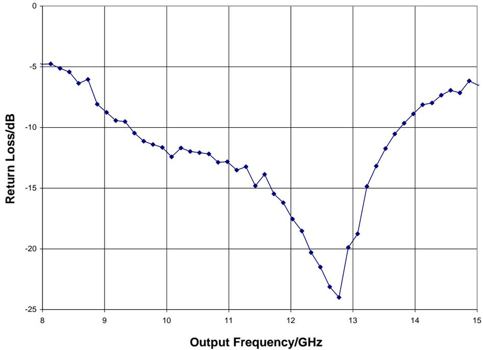
**Output Return Loss @ +15 dBm Drive Level,  $F = 11.5$  GHz Input,  $T_A = 25^\circ C$**
