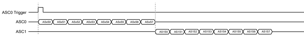
Figure 17-5. ASCx, ADCCTL.ADCMODE = 011b, 110b
