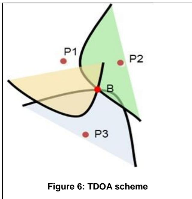
As shown in Figure 6 a tagged object (B) transmits a message that is received by all the readers (P1, P2 and P3 in the diagram shown here). Because radio waves travel at a constant speed, depending on the position of the tagged object, the message will arrive at some of the anchors before others. The time of arrival of the message at each reader is noted by the reader.
