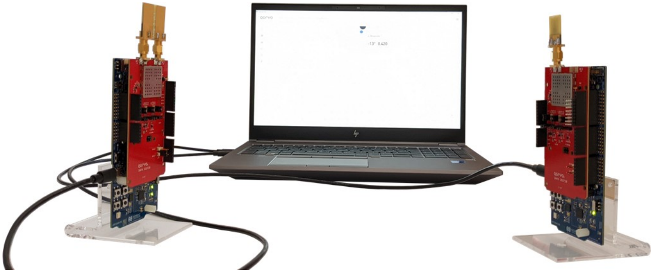
Fig. 1.3: QM33120WDK1 evaluation set-up
