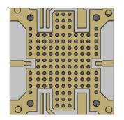
Figure 1. Mounting detail for the TGA2307-SM EVB PCB.
