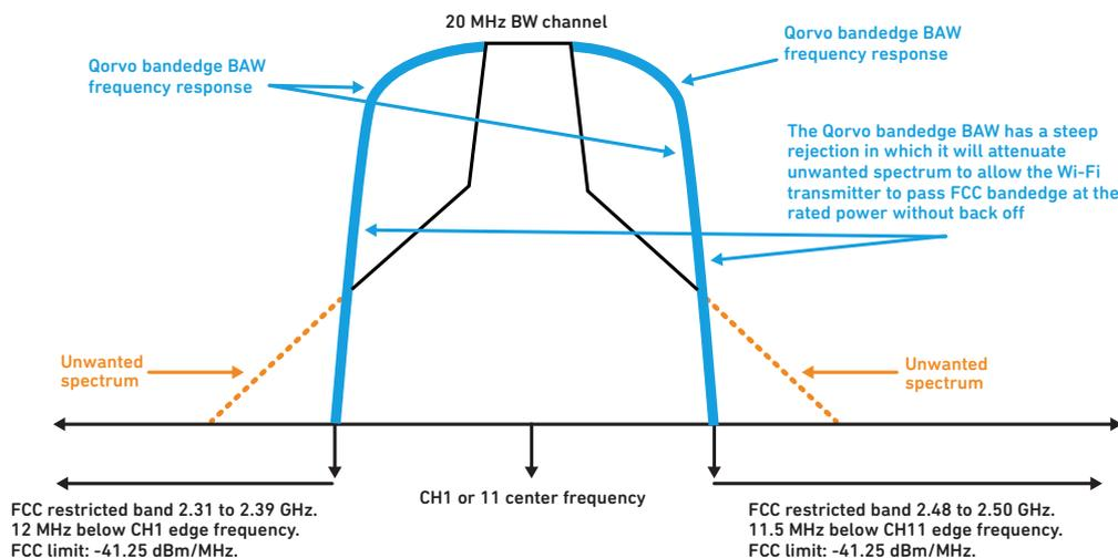
The use of the Qorvo bandedge BAW filters has proven to increase channel 1 & 11 output power by at least 10 dBm. This tremendously improves the range and the capacity of the Wi-Fi system.
