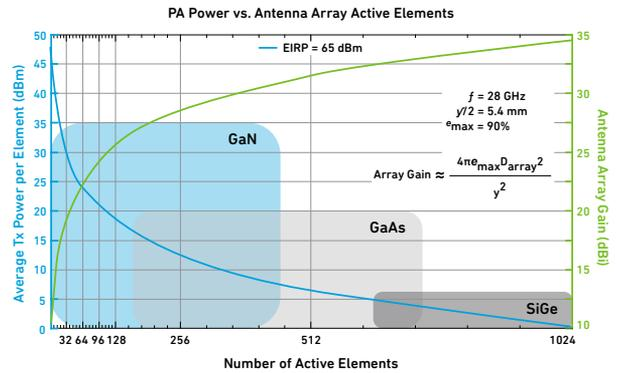
**Figure 15** Optimum RFFE technology vs. array size.
