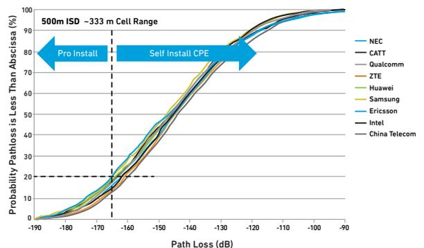
**Figure 5** Statistical path loss simulation for urban-macro environment with 500 m ISD.
