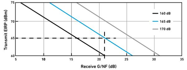
**Figure 6** Transmit EIRP and receive G/NF vs. path-loss for 1 Gbps edge-of-coverage throughput.
