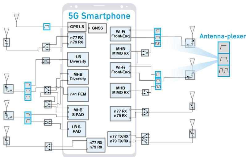
The number of bands in 5G use cases will continue to grow. The mobile device market has used SAW, BAW and FBAR filter technologies for decades. However, 5G will alter the allotted spectrum in mobile and non-mobile devices like handsets, Wi-Fi, automotive V2X, radar and infrastructure and presumably others not yet known. With all the possible 5G applications, discrete and integrated BAW will help engineers resolve complex antenna systems and coexistence challenges.
