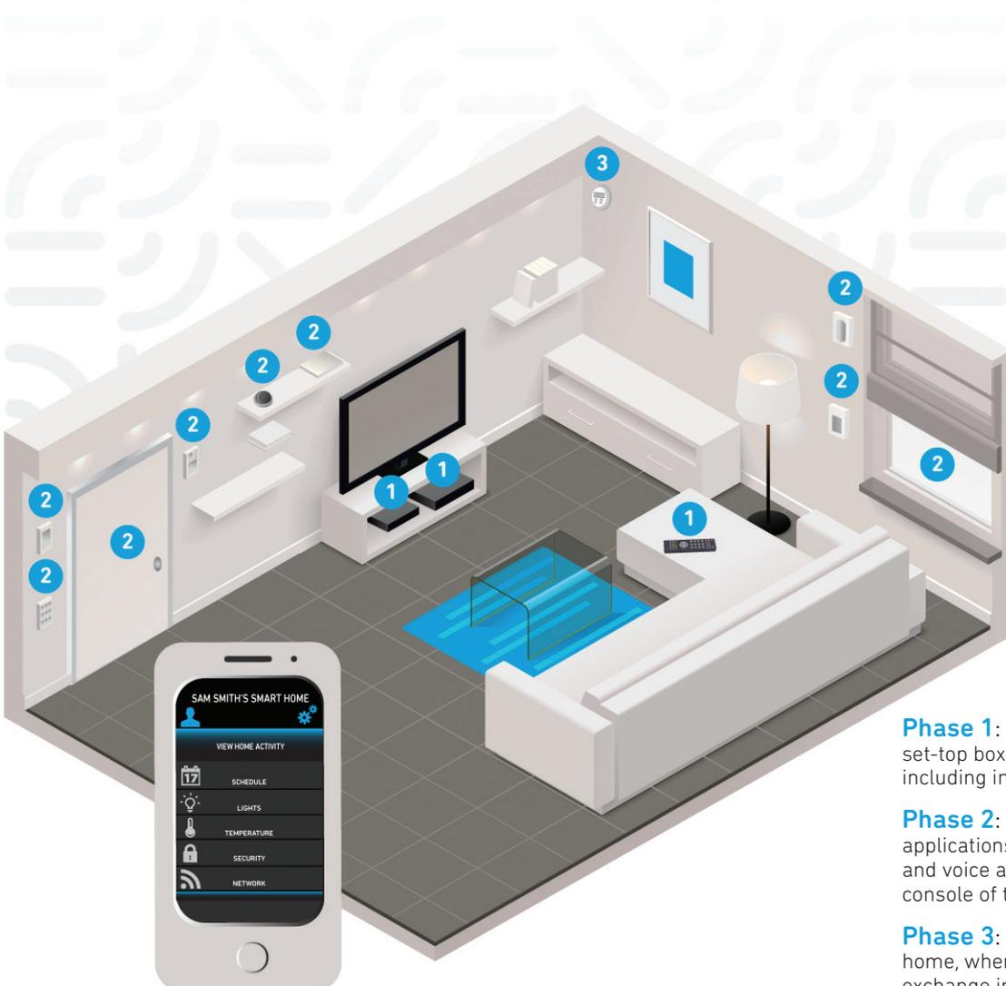
**Phase 1:** RF-based remote controls for set-top boxes and consumer electronics, including internet connectivity.
