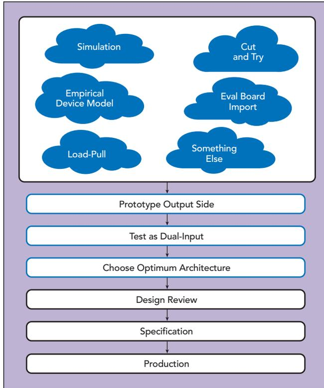
▲ Fig. 5 Measurement-aided design flow for a digital Doherty amplifier.
