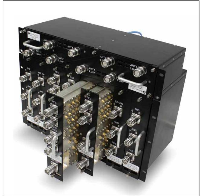
▲ Fig. 3 Neutral host small cell and D-RAN systems support several operators and must handle multiple carriers operating on different frequency bands.
