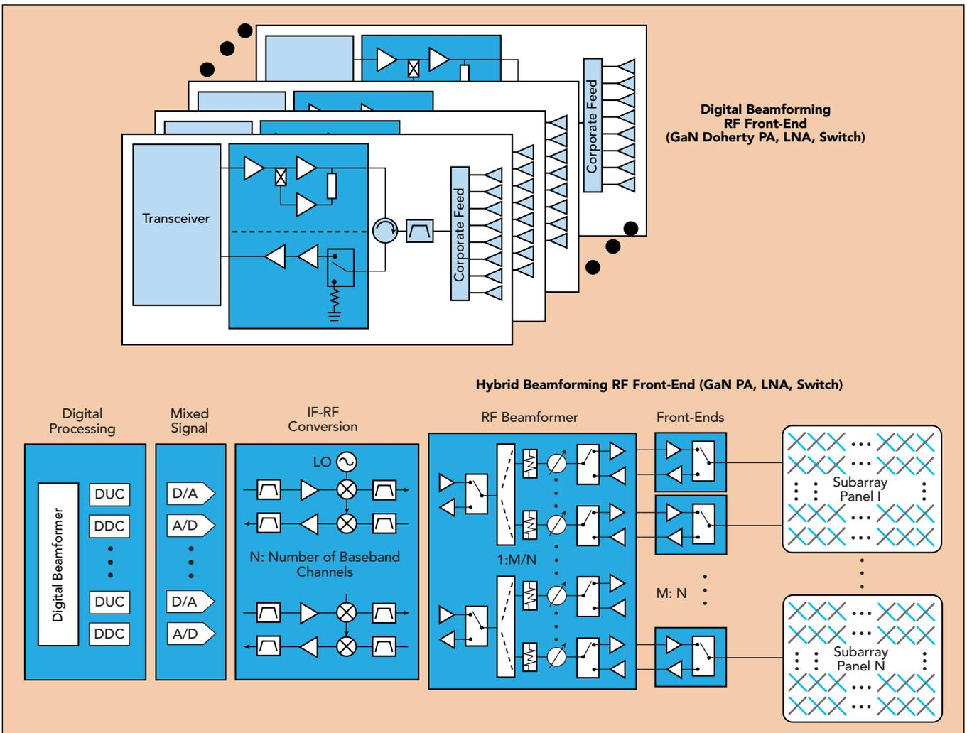
▲ Fig. 3 Digital and Hybrid RF Front-End Approaches.
