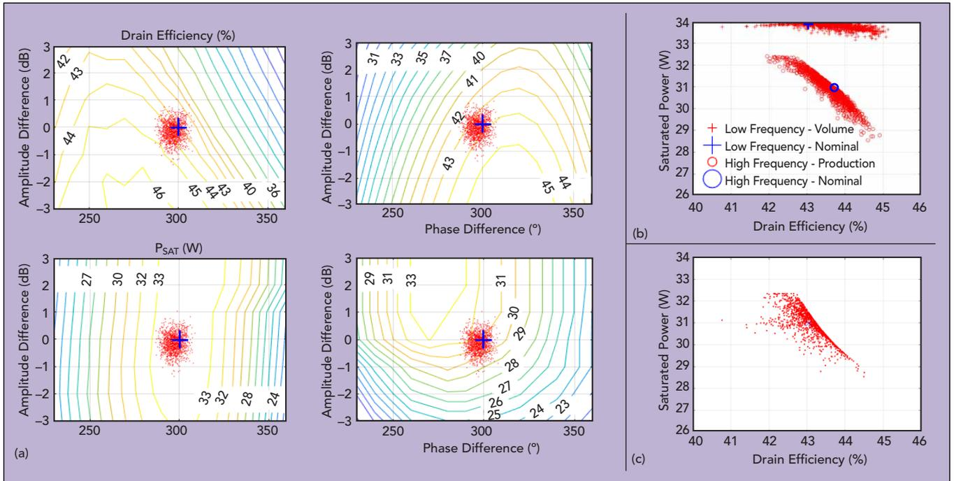
▲ Fig. 8 Gain and phase variation of a population of split digital Doherty amplifiers with a fixed RF input (a), saturated power and efficiency using a look-up concept (b) and cumulative, worst-case production distribution (c).
