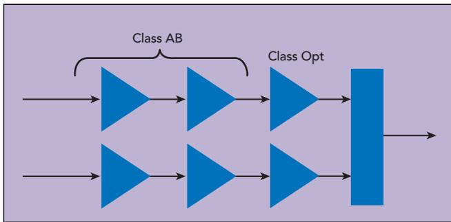
▲ Fig. 4 Digital Doherty amplifier, where the main and auxiliary amplifier operating class is digitally controlled.
