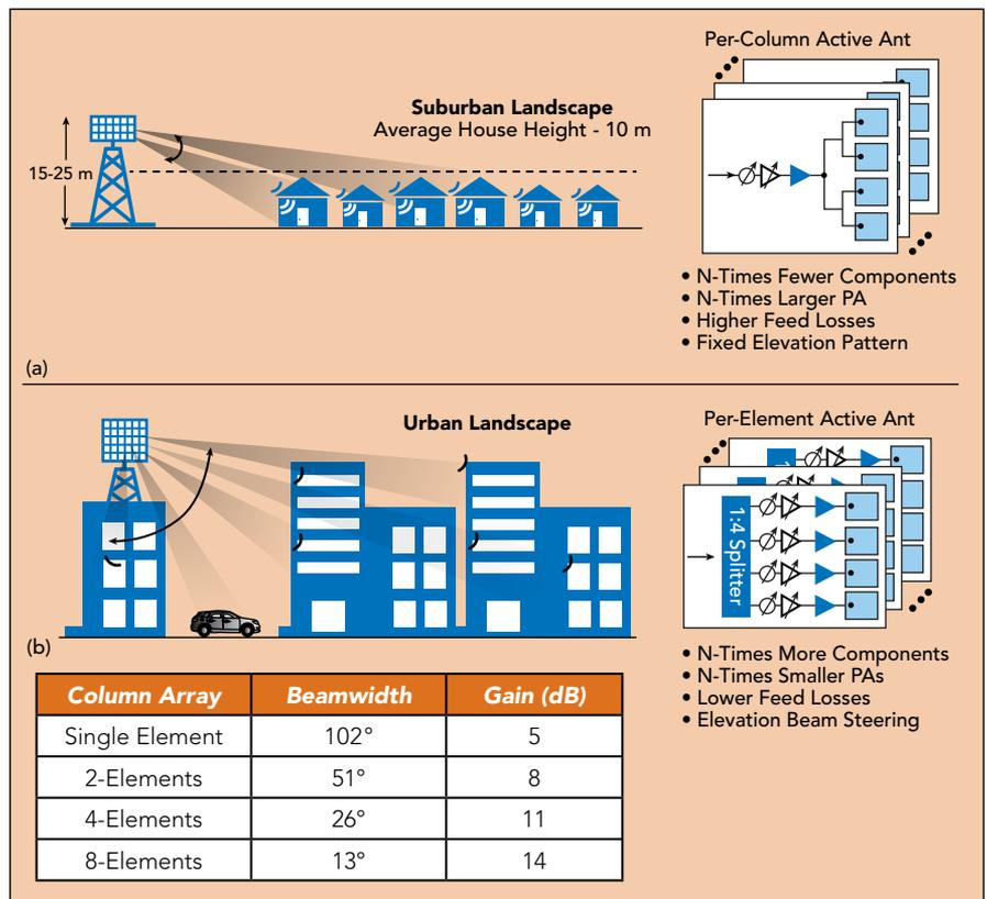
▲ Fig. 2 Array Complexity Depends on the Scanning Range Needed for the Deployment Scenario.
