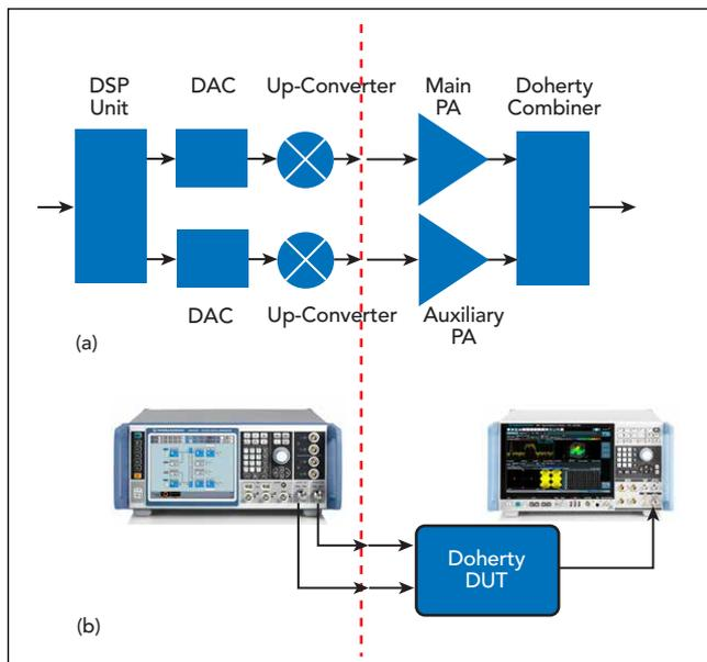
▲ Fig. 6 Simplified block diagram (a) and hardware setup (b) for designing a digital Doherty amplifier.
