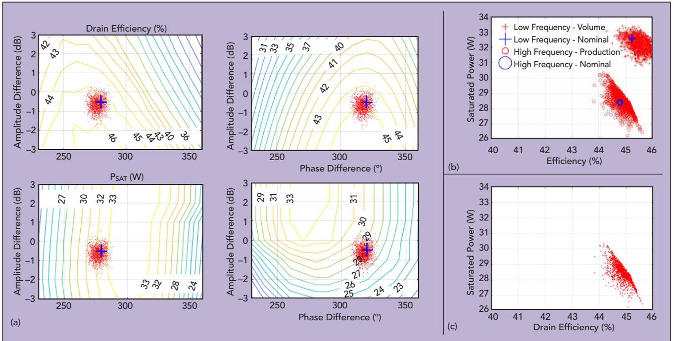
▲ Fig. 9 Digital Doherty amplifier population using a dispersive input split: gain and phase variation (a), saturated power and efficiency (b) and cumulative, worst-case production distribution (c).
