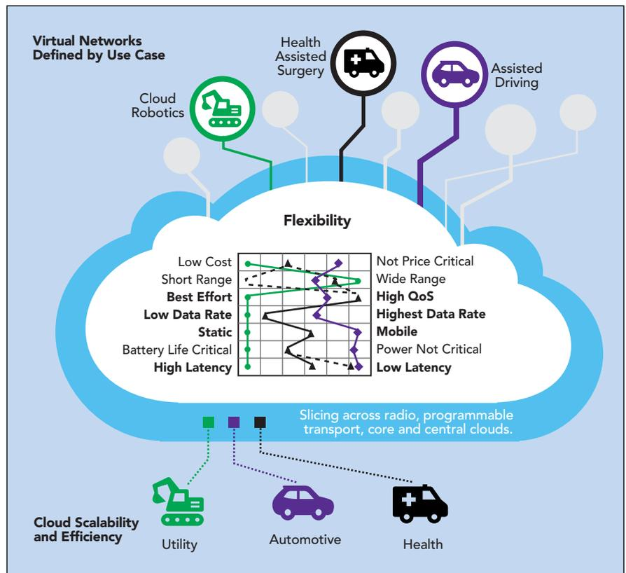
▲ Fig. 4 Using network slicing across the radio, transport, core and central clouds, 5G has the flexibility to support diverse use cases with a common underlying infrastructure.
