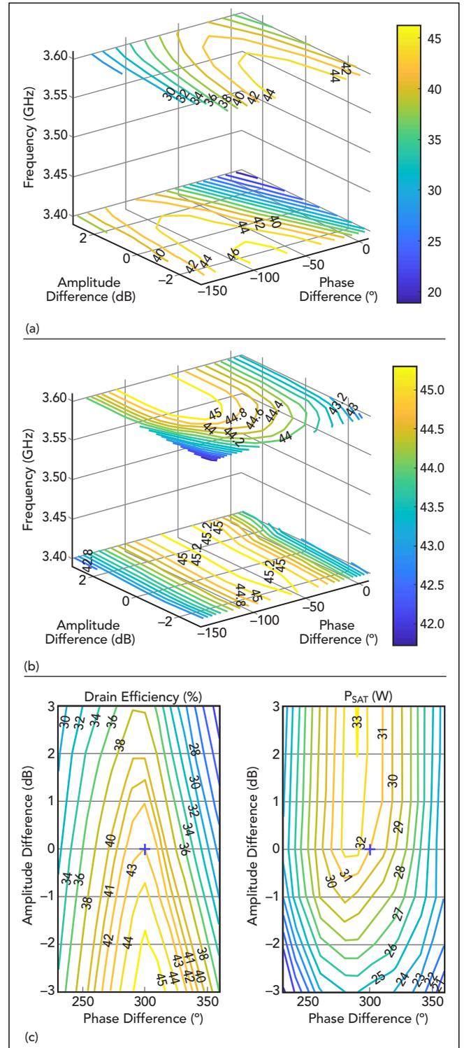
▲ Fig. 7 Dual-input Doherty in linear operation: measured efficiency at 35.5 dBm (a), saturated power (b) and worst-case efficiency and power (c).
