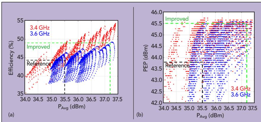
▲ Fig. 10 Efficiency vs. average output power (a) and PEP vs. average output power (b) for a dual-input Doherty amplifier using with square-law shaping and randomized phase.
