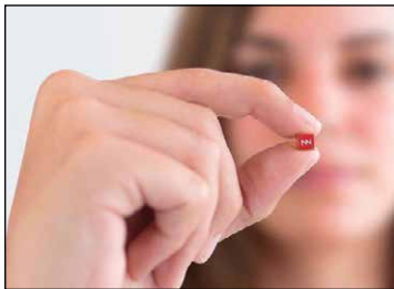
▲ Fig. 9 The CUBE mXTEND™ antenna booster from Fractus Antennas (5 mm 3 ).
