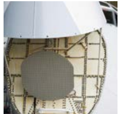
Phased array and AESA radar systems are being retrofitted into both commercial and military aircraft. They employ dozens of low noise amplifier MMICs that are relied on for receiver sensitivity and optimal SNR.
