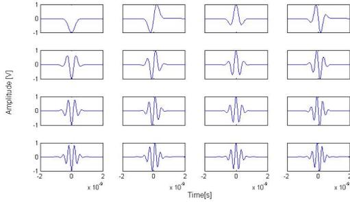
Fig. 2: The Gaussian pulse and its derivatives
