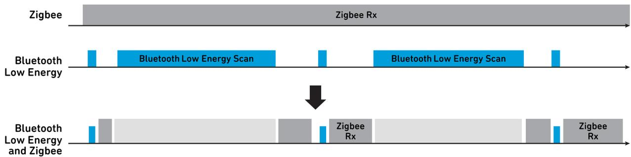
ConcurrentConnect technology is based on unique hardware features in Qorvo's platform that enable detection and identification of the packet in the most efficient way. Once detected, the packet goes through an identification process in real time on the hardware level, and then sends the packet to the appropriate protocol stack, eliminating the need for additional, non-real-time routing logic on the higher software layers.
