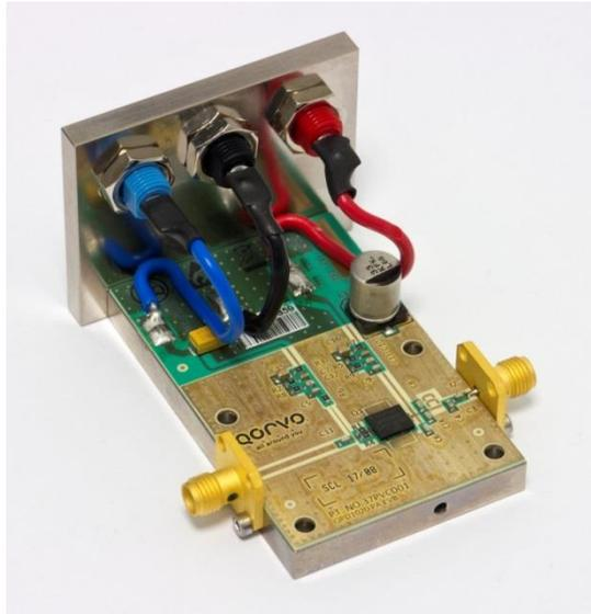
**Figure 7: Photograph of the QPD1020 PA Reference Design**
