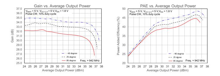
Test conditions unless otherwise noted: V<sub>BIAS</sub> = 5 V, V<sub>CC1,2,3</sub> = 5 V, V<sub>EN</sub> = 1.8 V, tested at 942 MHz using a pulse signal, 10% duty cycle.
