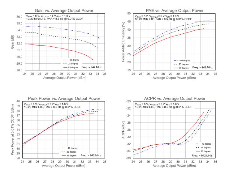
Test conditions unless otherwise noted: V<sub>BIAS</sub> = 5 V, V<sub>CC1.2.3</sub> = 5 V, V<sub>EN</sub> = 1.8 V, tested at 942 MHz using a single-carrier, 20 MHz LTE signal with 8.5 dB PAR at 0.01% CCDF on a reference design fixture.
