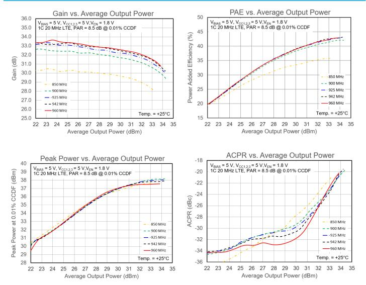
Test conditions unless otherwise noted:  $V_{BIAS} = 5 V$ ,  $V_{CC1,2,3} = 5 V$ ,  $V_{EN} = 1.8 V$ ,  $T = +25^{\circ}C$ , tested using a single-carrier, 20 MHz LTE signal with 8.5 dB PAR at 0.01% CCDF on a reference design fixture.
