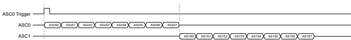
Figure 17-5. ASCx, ADCCTL.ADCMODE = 011b, 110b
