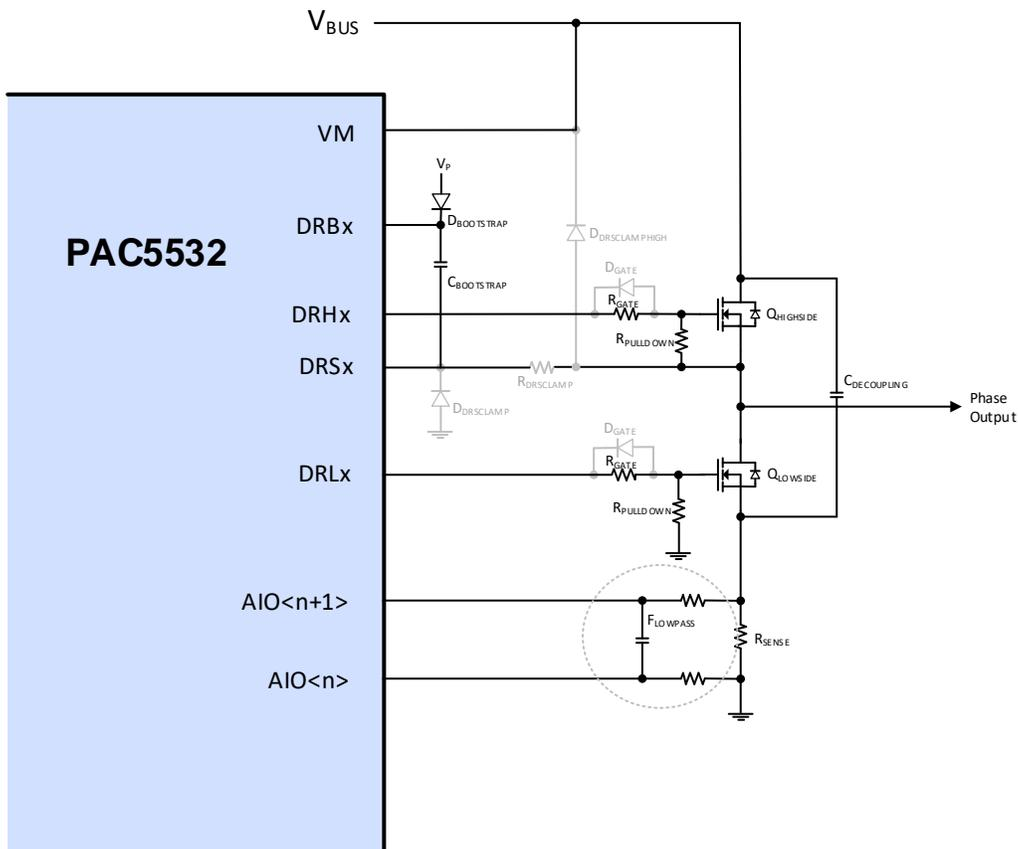
As the current load increases, voltage transients on DRS also can increase. These transients typically happen during the dead-time, when the current must find an asynchronous path to continue flowing.
