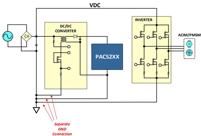
As an example, in the PCB layout shown below you can see from the diagram below how the three grounds are connected in a star at the DC/DC bus capacitor.
