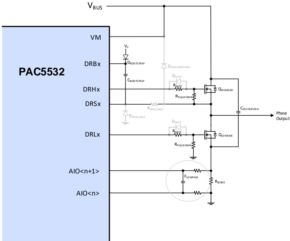
Some of the PAC552X low-voltage (< 70V) devices have a small tolerance for negative-going voltage on the DRS node, so this diode helps prevent this situation.
