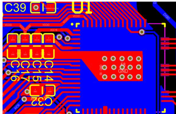
In the example above, the IC has a ground pin that is used for the copper polygon connecting the bypass capacitors to the power pad. The power pad has several vias to the ground plane to decrease impedance to the ground plane.
