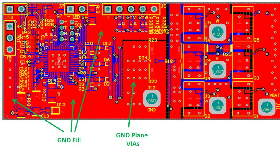
As shown in this layout, available area on the top and bottom layers (red and blue, respectively) is filled with copper for ground. These ground planes are connected with vias to maximize the benefit of the overall ground plane on both layers.
