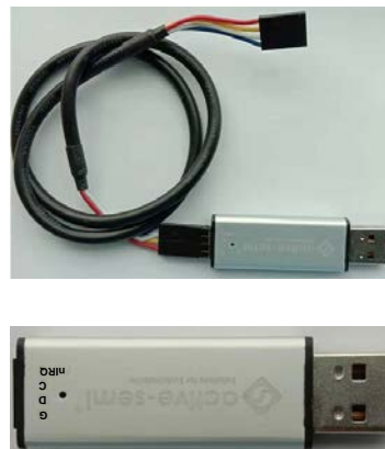
Figure 4 – USB-TO-I2C Dongle Connection
