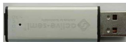
Figure 4 – USB-TO-I2C Dongle Connection
