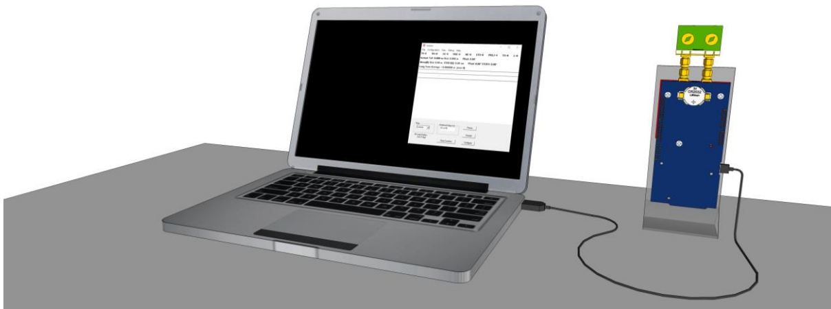
Figure 12 - Connect the NODE to the PC and start DecaRanging-PC
