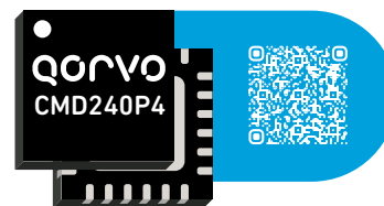
DC-22 GHz Distributed Driver Amplifier MMIC Gain 15 dB P1dB 19 dBm NF 2.2 dB 4x4mm QFN
