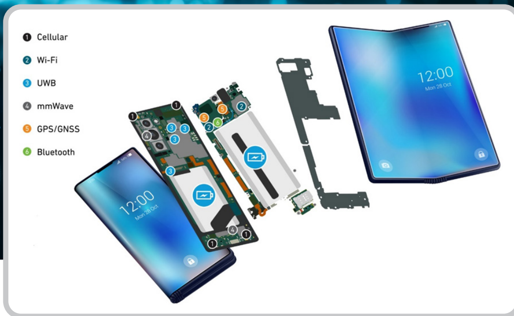
Figure 1: As manufacturers add more non-cellular bands to provide faster networking and support new location-based services, RF challenges continue to increase. (Source: Qorvo)
