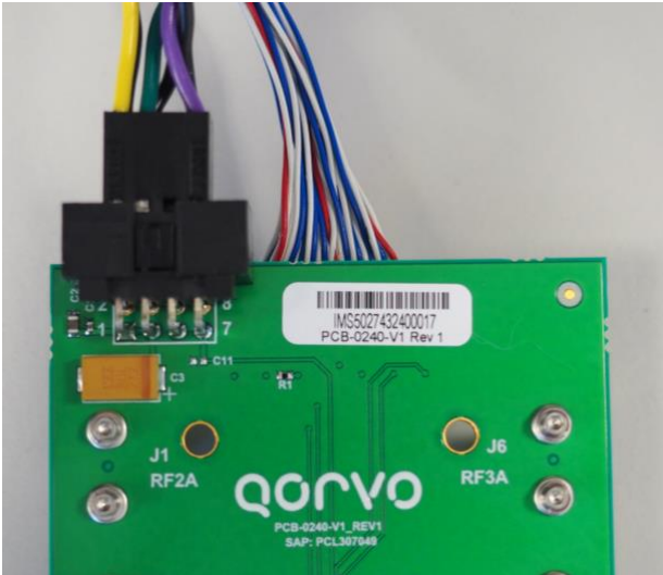
Figure 22: Top side view: Power cable connected to P2
