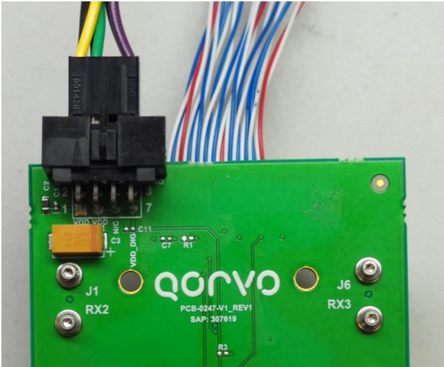
Figure 21: Top side view: Power cable connected to P2
