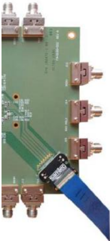
Figure 19: Connect IO Cable to P1 on Evaluation Board
