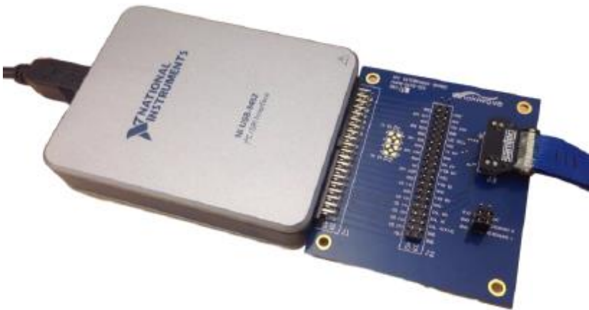
Figure 20: Connect IO Cable to P3 on Interposer Board
