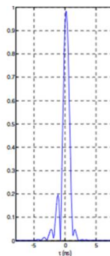
Fig. 2-3. Example of UWB nanosecond wide pulse signal
