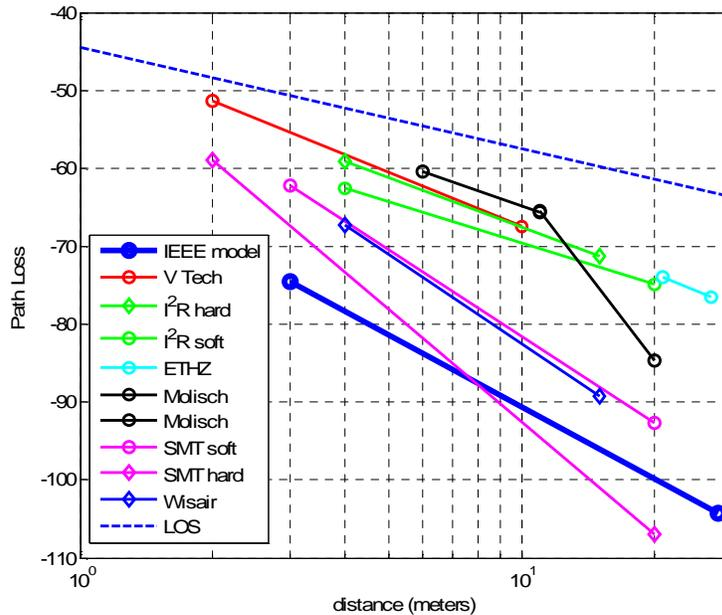
Figure 1. Different path loss models for UWB channels
