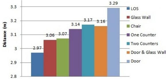
Fig. 10: Ranging Results of Soft-NLOS Area at 3m Point
