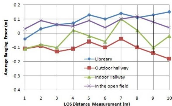
Fig. 9: Ranging Results of LOS Area Measurement
