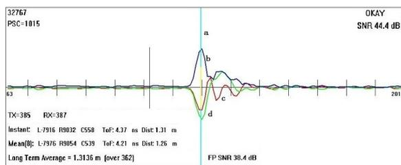
Fig. 7: Received UWB Signal Response
