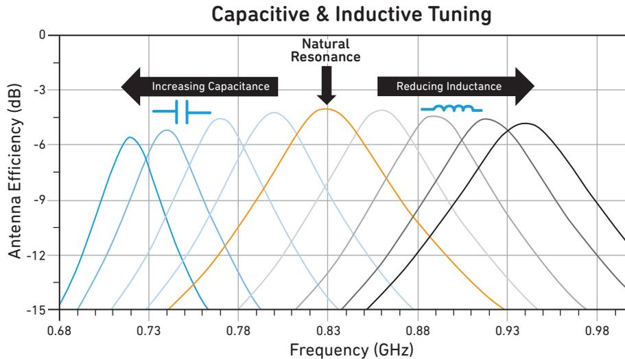
Tuning location A vs B (closer to the feed vs closer to the open end)
