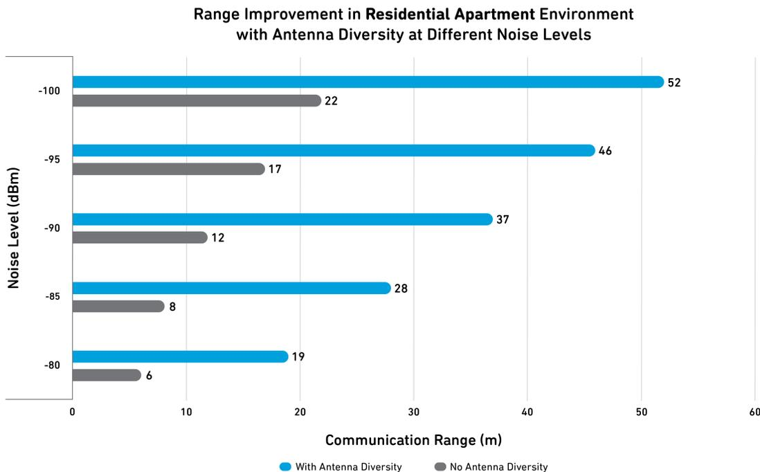
Figure 5: Communication range between QPG6105 and QPG7015M with and without antenna diversity (residential apartment environment).
