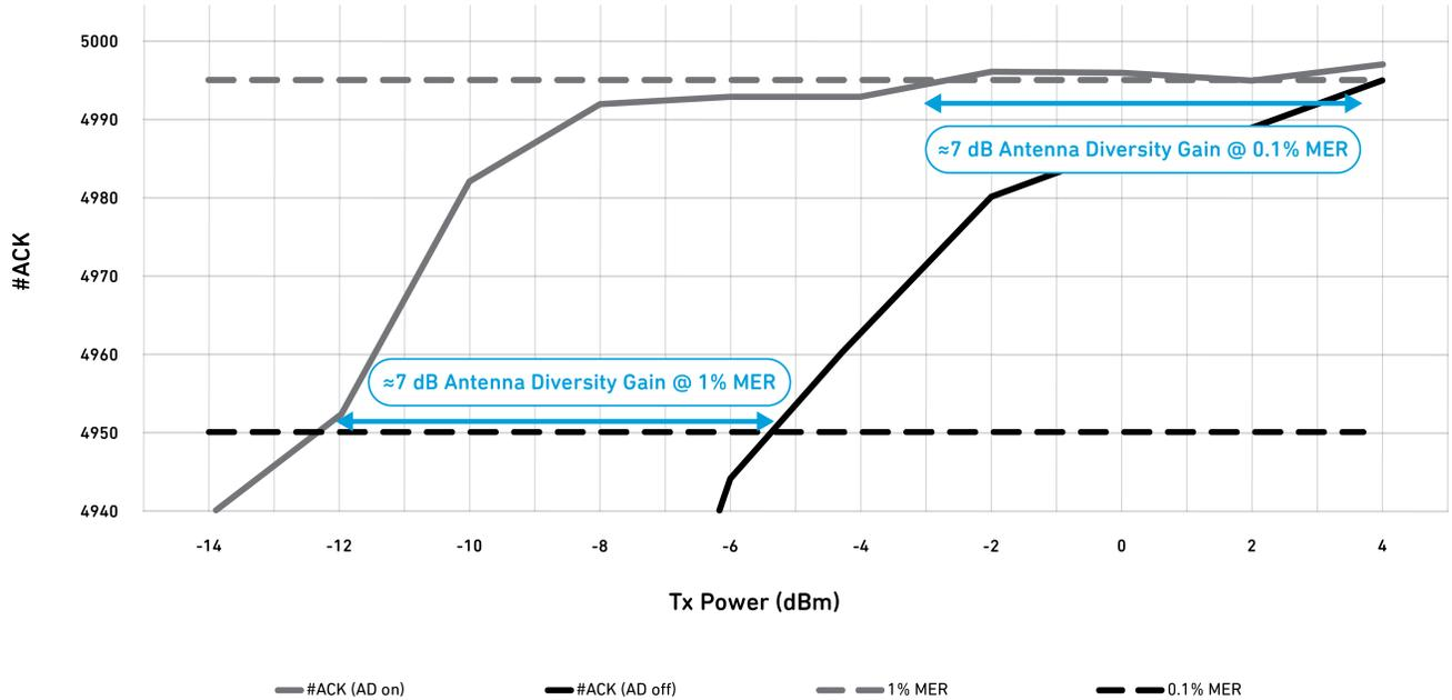
Figure 8: Range test with and without Rx antenna diversity.
