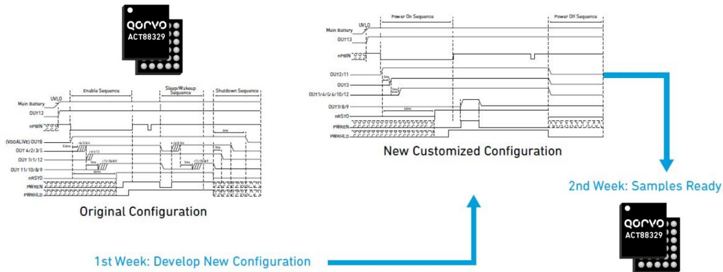
**Figure 4:** Designers can assess performance with various parameter configurations and then easily reconfigure them for optimized performance using a Qorvo-supplied GUI and a PC linked to an ACTIVECiPS™ PMIC. (Source: Qorvo).
