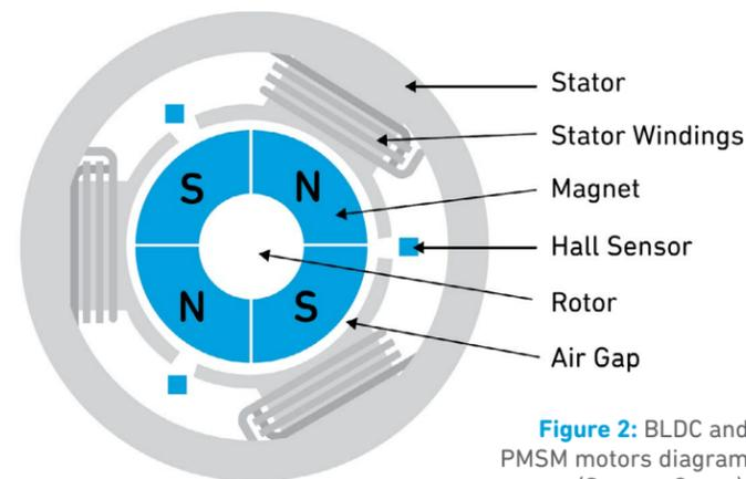
Figure 2: BLDC and PMSM motors diagram (Source: Qorvo).
