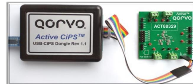
**Figure 6:** ActiveCiPS™ Dongle enables you to debug your design and change the PMIC default settings on your boards on the spot. (Source: Qorvo).
