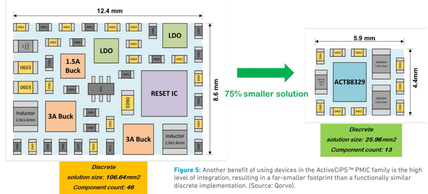
**Figure 5:** Another benefit of using devices in the ActiveCiPS™ PMIC family is the high level of integration, resulting in a far-smaller footprint than a functionally similar discrete implementation. (Source: Qorvo).
