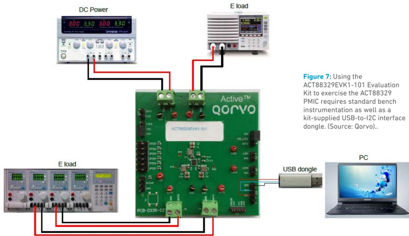
**Figure 7:** Using the ACT88329EVK1-101 Evaluation Kit to exercise the ACT88329 PMIC requires standard bench instrumentation as well as a kit-supplied USB-to-I2C interface dongle. (Source: Qorvo)..
