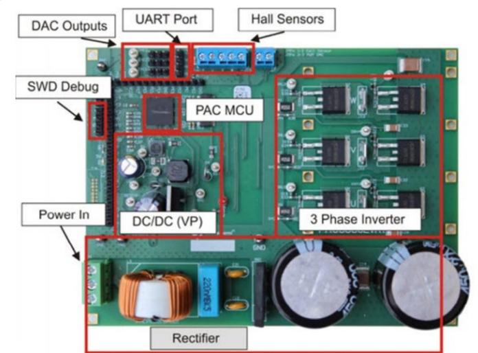
**Figure 3:** The Qorvo PAC5556EVK1 evaluation board. (Source: Qorvo)
