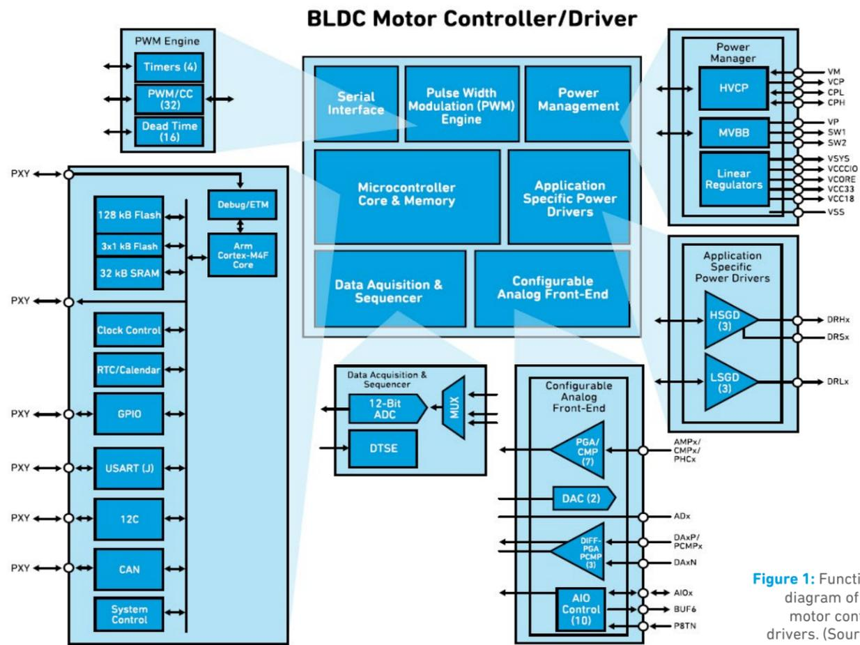
**Figure 1:** Functional block diagram of the PMSM motor controller and drivers. (Source: Qorvo).
