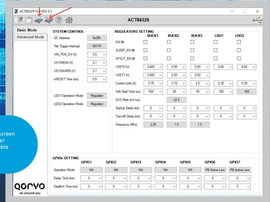
**Figure 9:** A subsequent screen of the GUI provides further insight into the configurable options. (Source: Qorvo).
