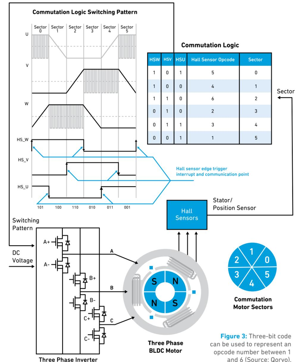
Figure 3: Three-bit code can be used to represent an opcode number between 1 and 6 (Source: Qorvo).
