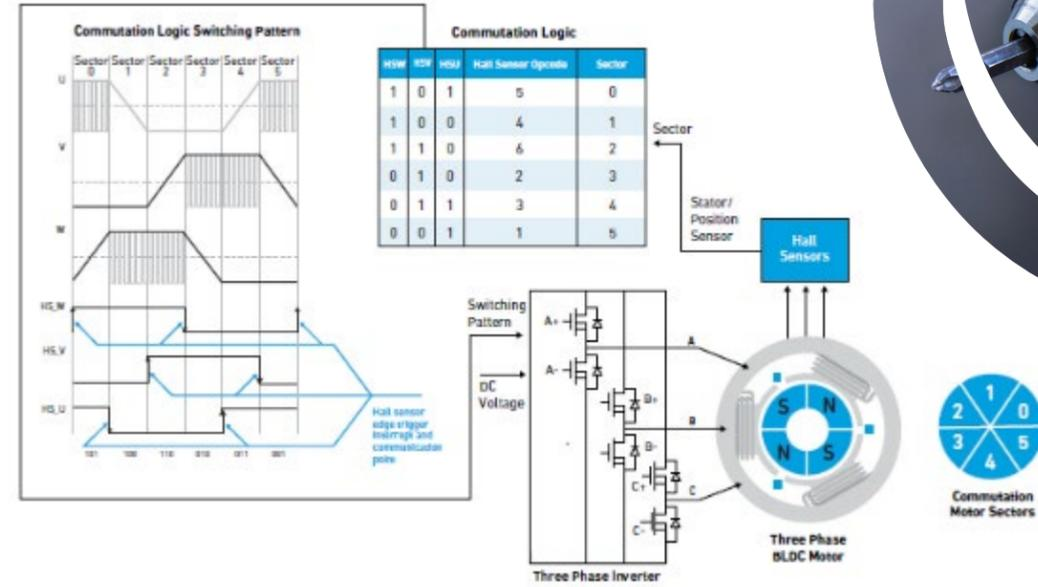
**Figure 3:** BLDC motors do not have a physical commutator and must use commutation logic sequencing. To obtain efficiencies, both magnetic fields must be aligned as perfectly as possible using a control circuit. (Source: Qorvo).
