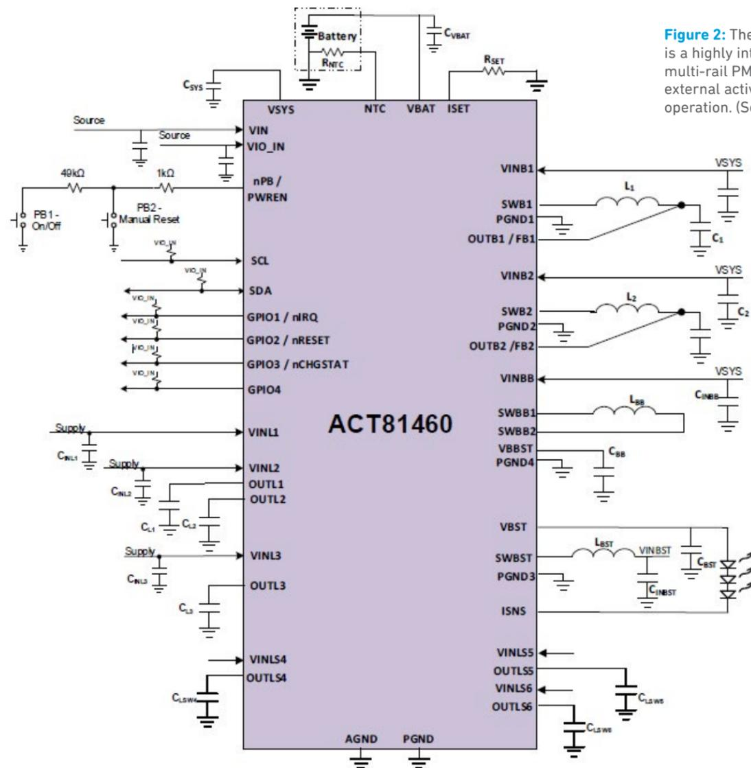
**Figure 2:** The Qorvo ACT81460 is a highly integrated, low-power multi-rail PMIC that requires no external active components for operation. (Source: Qorvo).
