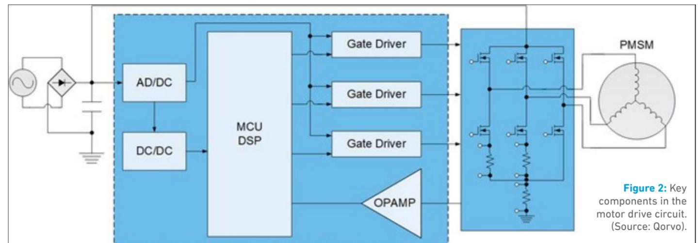
**Figure 2:** Key components in the motor drive circuit. (Source: Qorvo).
