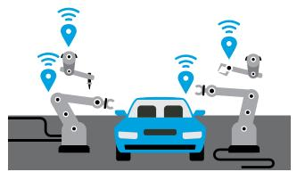
Location-based applications make use of the real-time accurate location data from UWB sensors for use cases targeted at locating and tracking objects.
