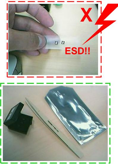
Do <u>not</u> use tape or other static-generating materials on or around devices.
