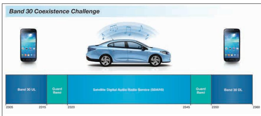
▲ Fig. 3 Band 30 and satellite radio service coexistence challenge.
