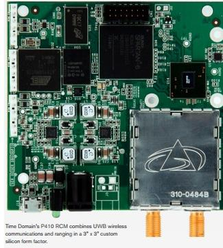
Figure 5.2: Time Domain real time location technology (P410) (from the Time Domain website : [www.timedomain.com/](http://www.timedomain.com/)).
