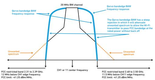
Figure 7: With Qorvo BAW filter: Steep frequency response profile at the bandedge helps to recover linear power on channel 1 and 11.
