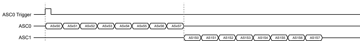
Figure 17-5. ASCx, ADCCTL.ADCMODE = 011b, 110b
