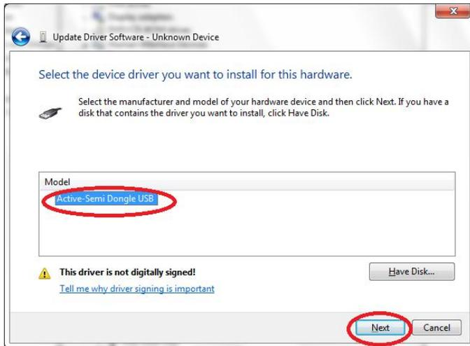
Click on **Active-semi Dongle USB** and then click **Next** button to start installing the driver
