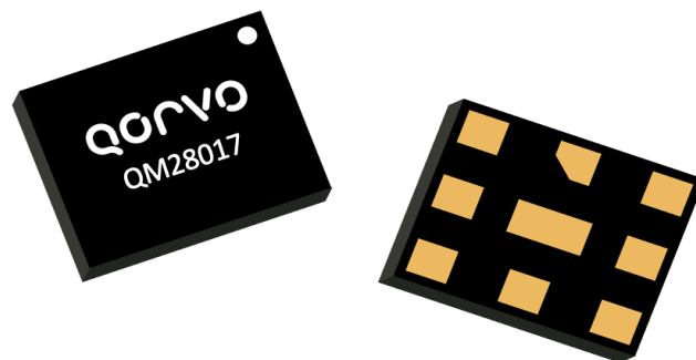
9 Pin 2.0mm x 1.6mm x 0.6mm leadless SMT package
