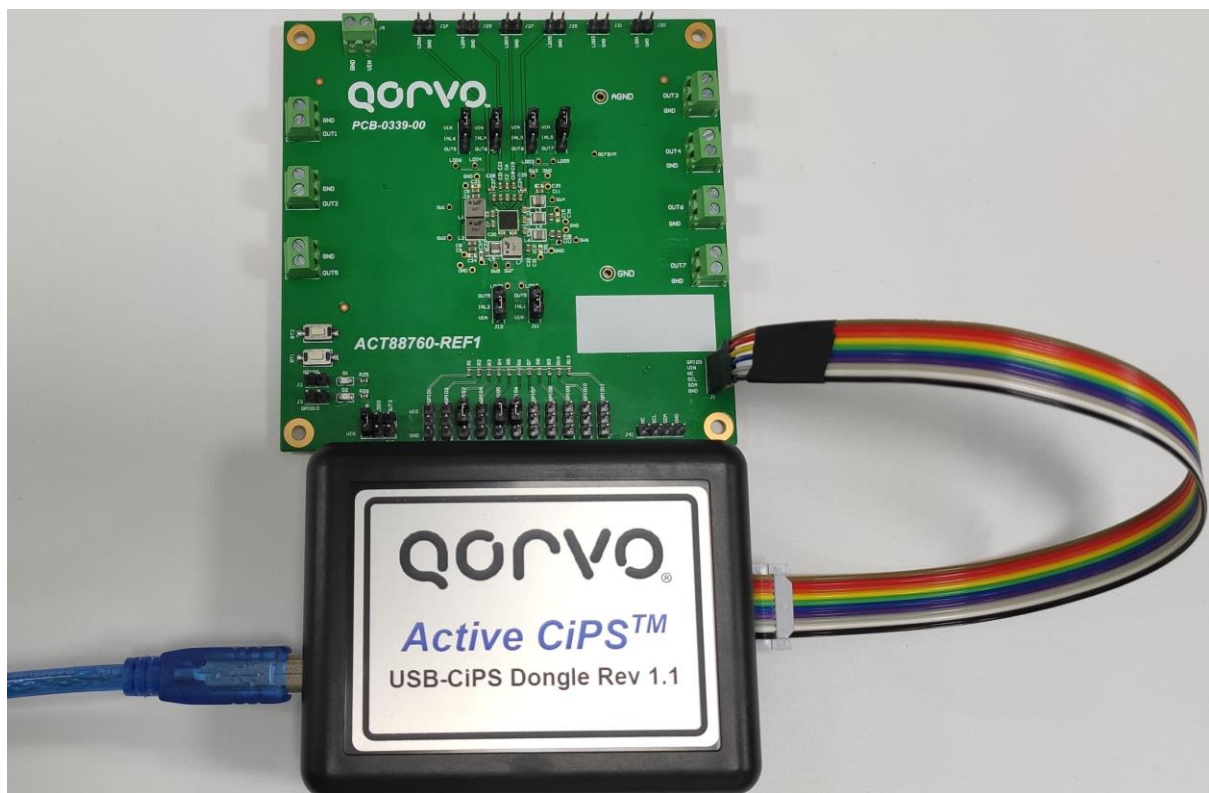
Figure 1: ACT88760 and ActiveCiPS™ Dongle Connection
