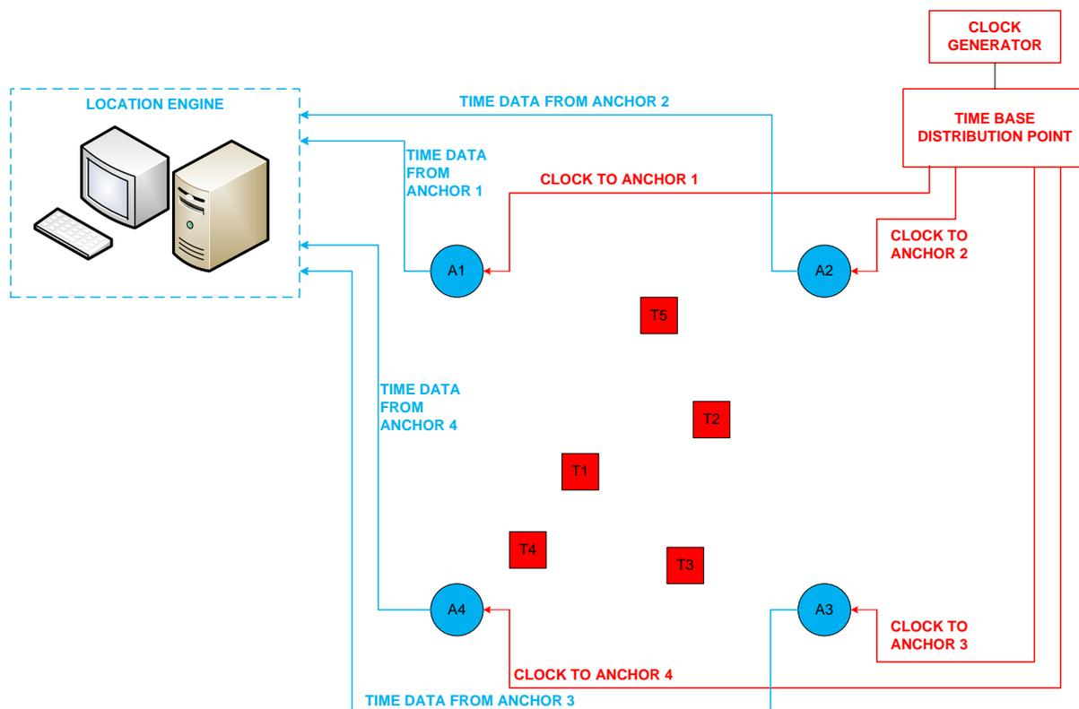
Figure 1: Basic concept of a wired synchronization scheme
