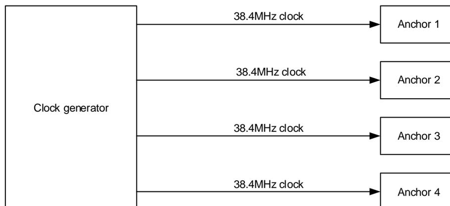
**Figure 2: Clock signal distribution**
