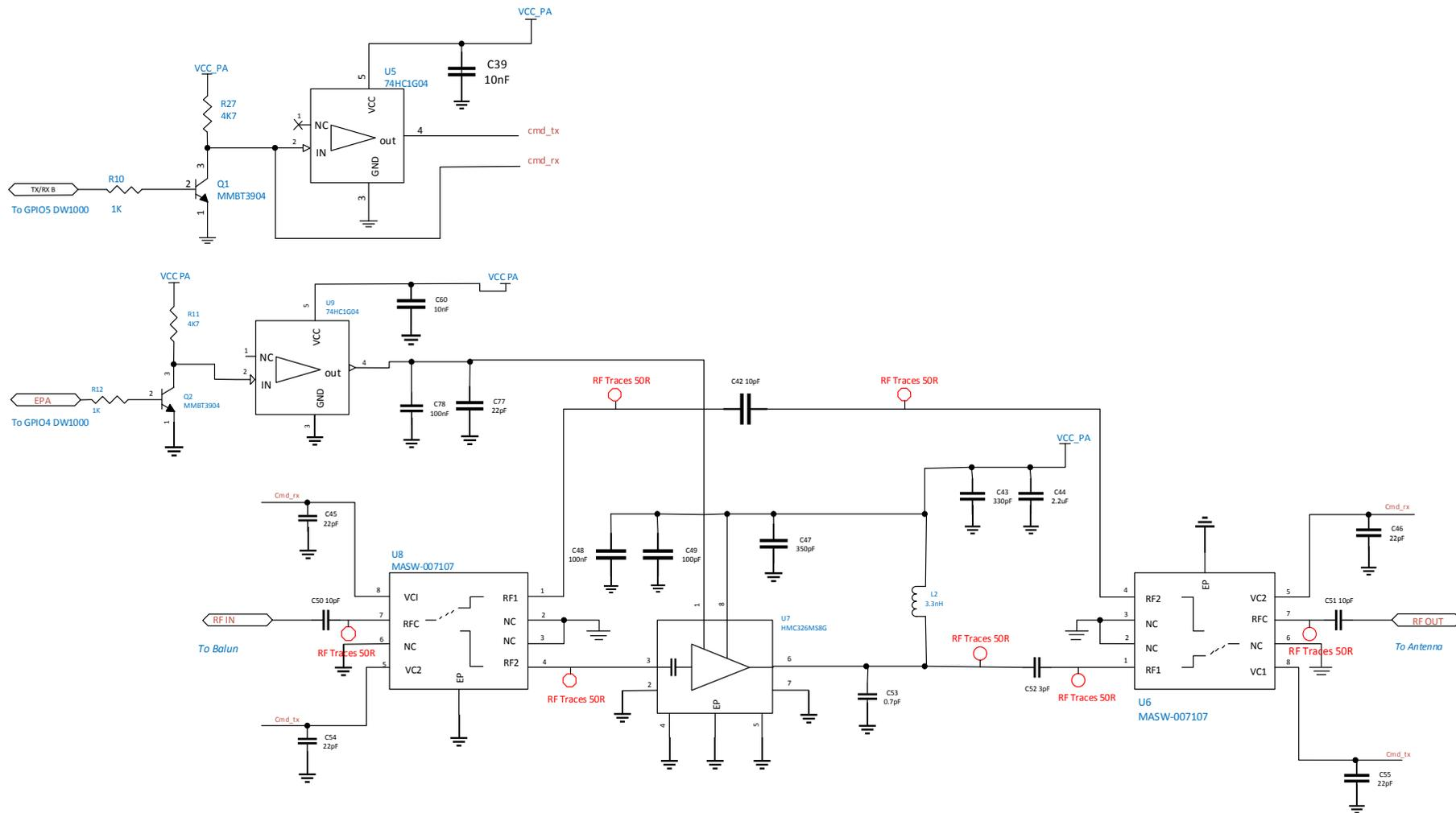
Figure 2. Hardware schematic
