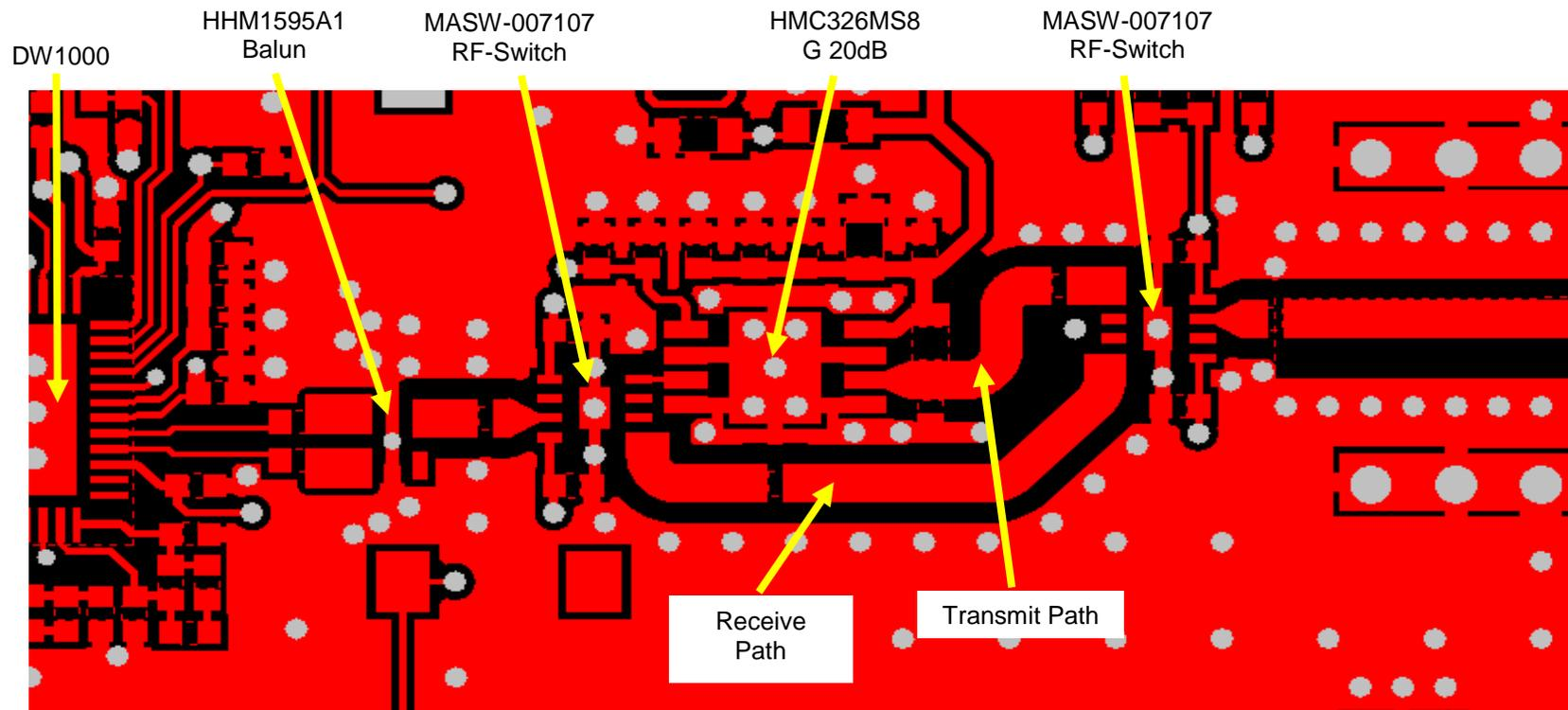
Figure 3: PCB Layout
